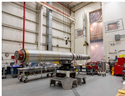
DEUCE on the mass properties measurement table. Photo by Berit Bland/NSROC
